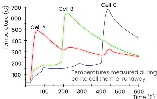
Figure 2. Cell to Cell Thermal Runaway - Immersion Protection
